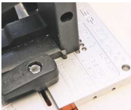
▲ Each style of joint has a set of indexing marks
